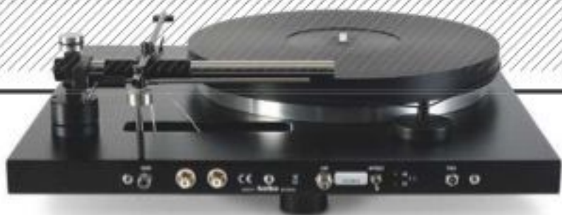
ABOVE: Connected via a soft 6\text{mm} PVC umbilical the 'Air' intake valve feeds both the platter and tonearm 'bearings'. Fine arm leads are terminated in gold-plated RCAs while 33.3/45 speeds are selected via a toggle and adjusted via two trimpots
